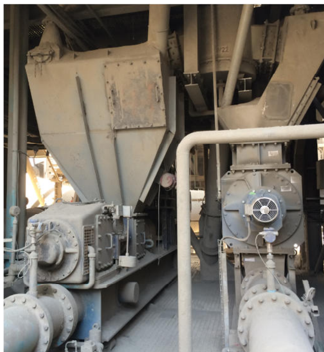
Image 2b: Stand-by pump (on the left) and new KREISEL rotary feeder (on the right) [after modification]
